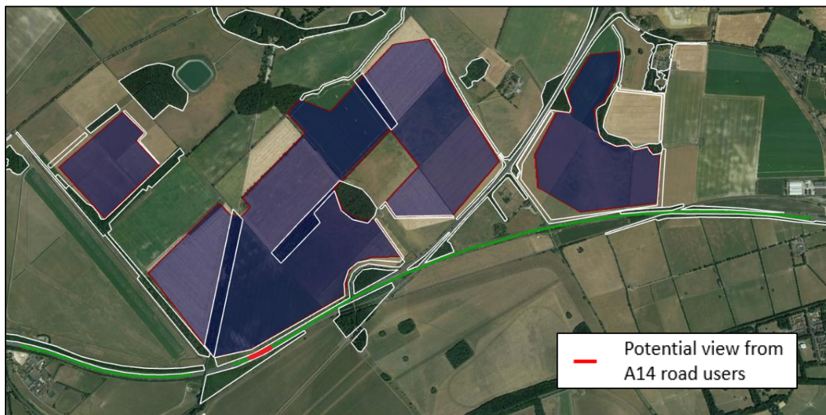
Plate 16-1 Potential for glint and glare from A14 for road users traveling in a south-westerly direction
